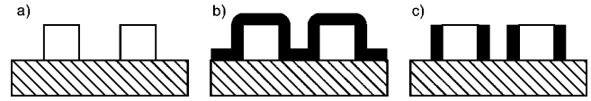
FIG. 2. Schematic representation of the essential steps in the filet process (cross section). (a) Definition of an array of SiO 2 bars on a p -Si layer (hatched area). (b) The bars are covered with a thin p -Si layer. (c) After anisotropic etching of the structure in (b) a thin sliver of p -Si material remains at the sidewall. The thickness of these slivers is equal (or at least proportional) to the thickness of the deposited layer. The slivers then serve as a mask for etching the underlying p -Si layer, and are much smaller than the originally patterned structure in (a).
